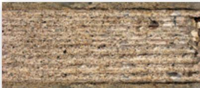
Equip the KR8HD with our standard carbide tip cutters for grinding, leveling, grooving, cleaning and general surface preparation. The standard carbide tip cutter is a very aggressive cutter designed for removing material fast.
