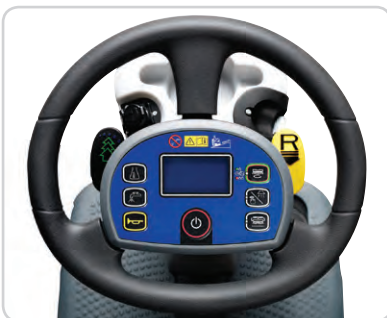
Extremely user friendly and easy to learn. Dashboard with One-Touch button and intuitive display integrated into the steering wheel.
