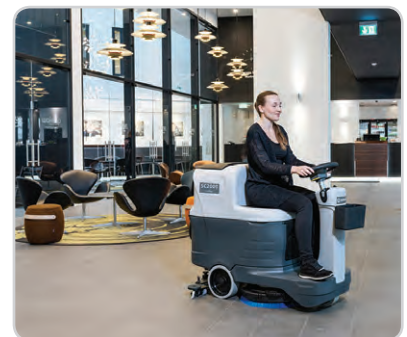
Quiet mode lowers the already quiet level of 68 dB A to an astonishing low 62 dB A.
